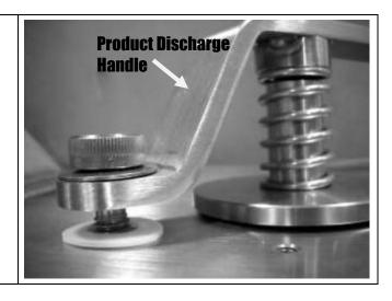
Press down on product discharge handle, ensuring the discharge cover and discharge handle are aligned with each other.
