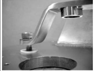
Assemble discharge cover, O-ring and spring.
